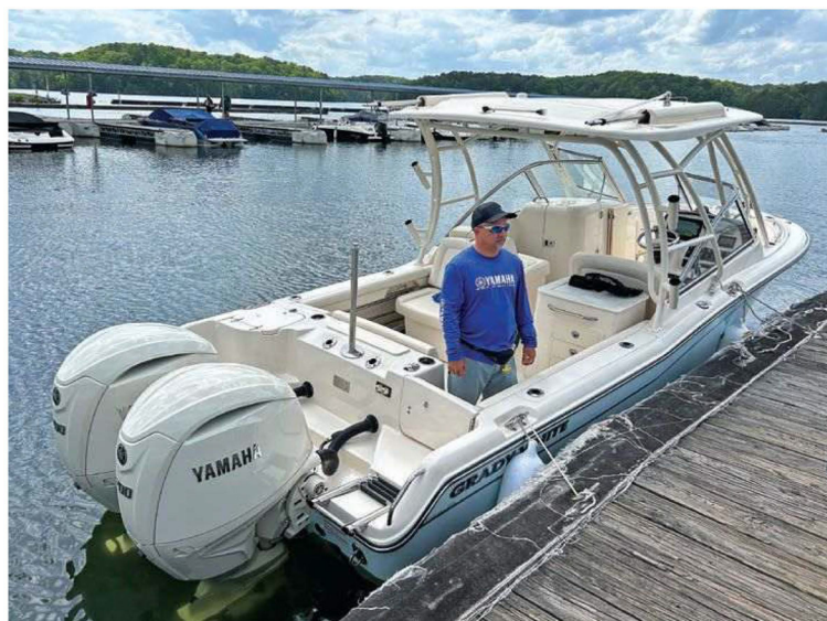
Left: The test boat, a Grady-White Freedom 255 dual console with twin 200-hp outboards. Above: The author takes the wheel to begin the controlled speed tow test.
