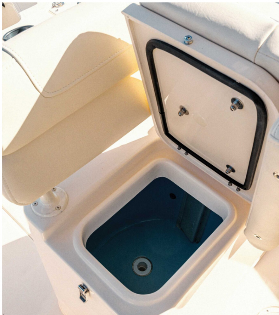
A 25-gallon livewell with a cover that seals tight to prevent splashing is integrated into the lean bar/seating module of the Grady-White 231 CE. Courtesy Grady-White
