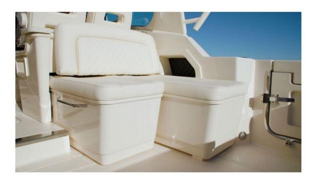
The aft facing seat can be extended into a lounge at the press of a button, or kept compact to retain cockpit fishing space. Photo via Grady-White.
