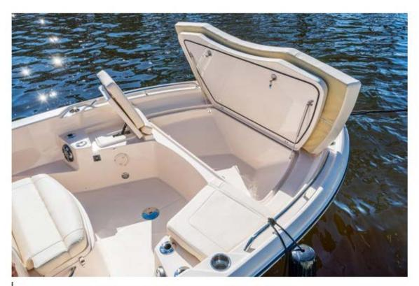
The 277-quart forward fishbox is insulated and drains overboard.
