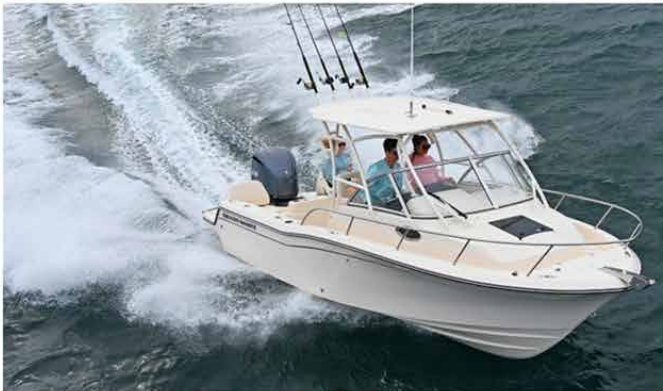
Note how the SeaV2 bottom design pushes spray out and down. Combined with lots of freeboard forward, this helps deliver a dry rider in most conditions.
