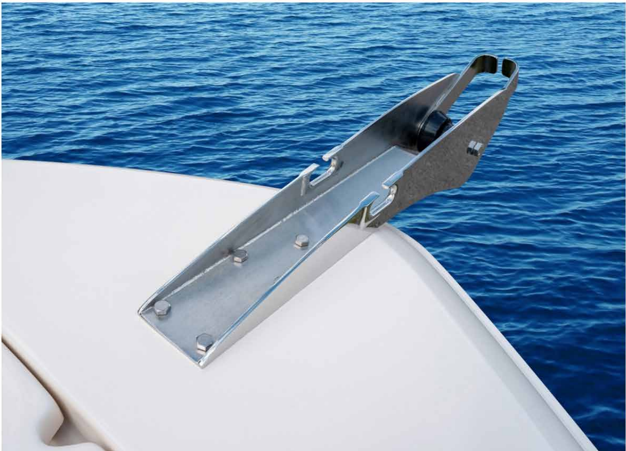
Bow Anchor Roller: This makes life a lot easier for the line-handler, particularly if it's you. Add a plow-style anchor and you're good to go. It also gives you a place to store an anchor, having it ready to go without having to dig it out of the locker.
