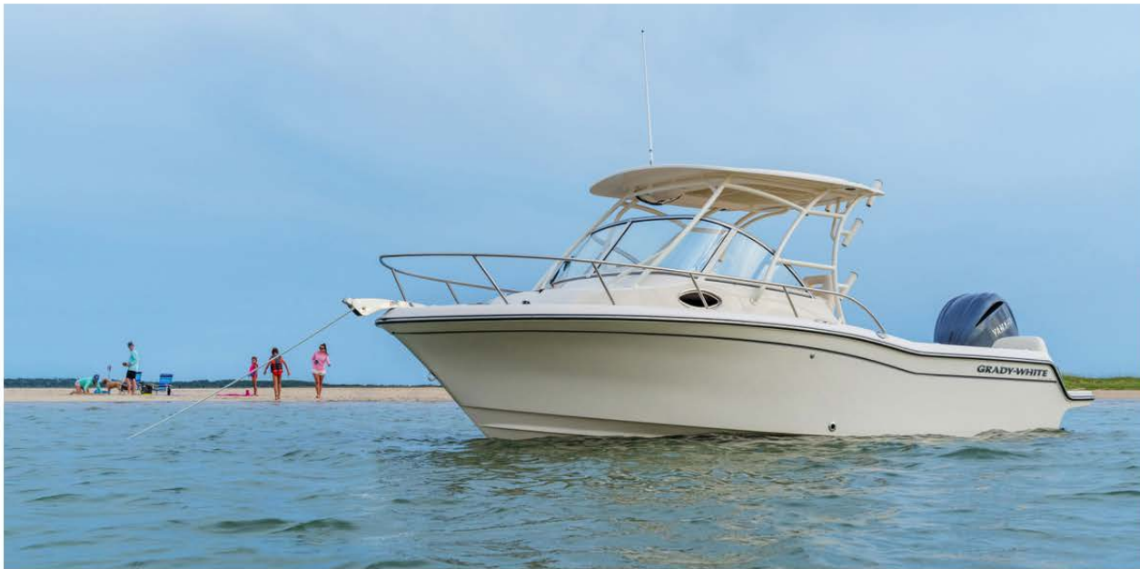
The sheer line seen here is a Grady-White trademark, as is the sharp forward entry of the SeaV2 hull. Note the molded in swim platforms.
