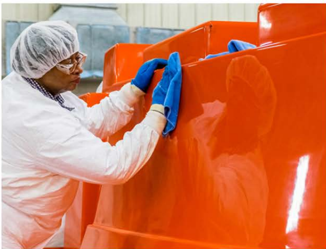
Molds are polished to a mirror finish before gelcoat is applied.
