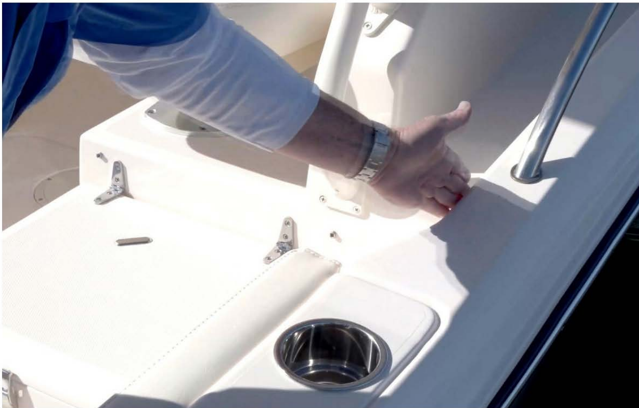
The walk-around to the bow is made easier by a narrowing of the bulwarks in this section of the cap rail.
