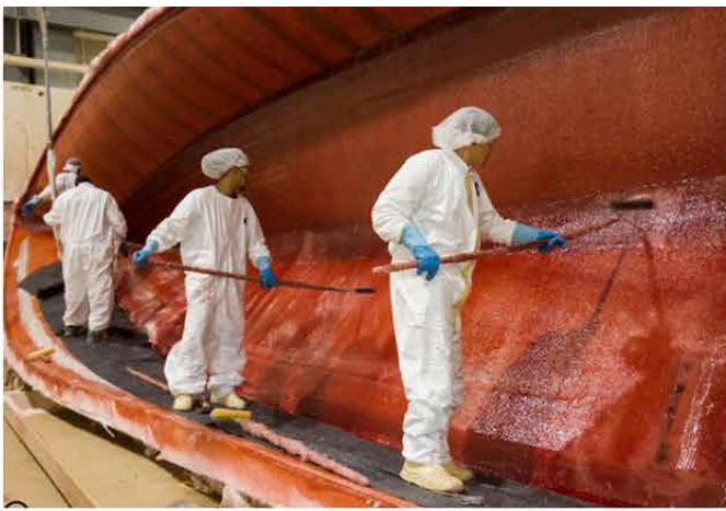
Lamination includes multiple layers of bi- and tri-directional fiberglass fabric.
