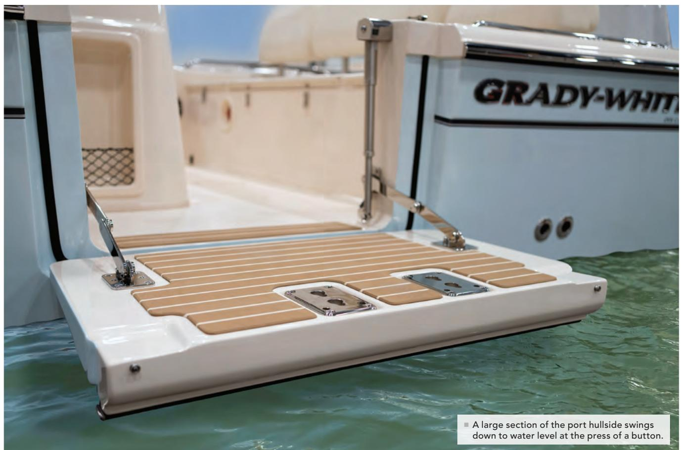
■ A large section of the port hullside swings down to water level at the press of a button.
