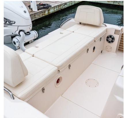
Full-width transom bench seating with pivoting backrests quickly converts to an abbreviated stern casting deck when it's time to start fishing.
