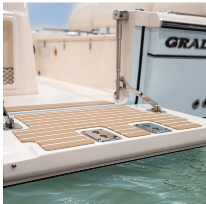
A portside door hinges downward at the touch of a button to haul aboard big fish or serve as a swim platform with a removable boarding ladder.
