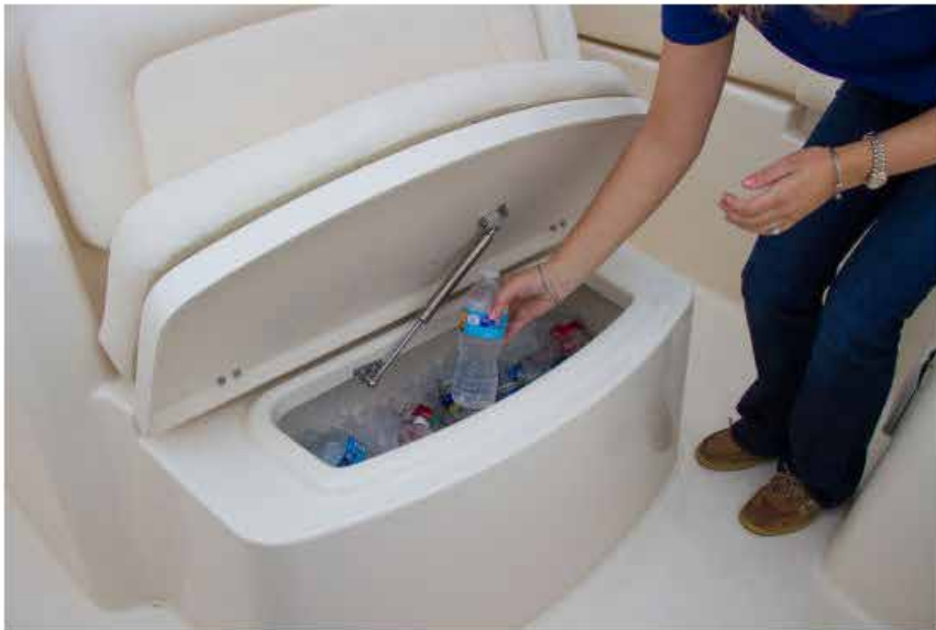
The seat box forward can be used for a number of different purposes. As you can see here, where it is used as an ice chest. It can also be a 67-quart fishbox. It drains overboard.
