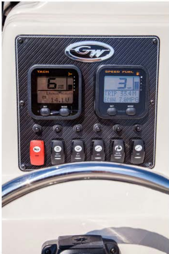
This GW panel includes information about engine functions, fuel levels and has lighted rocker switches and waterproof breakers.
