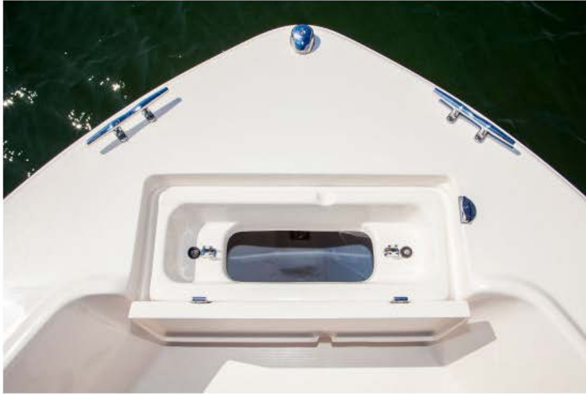
The anchor locker includes stainless steel clamps and rode storage. It can accommodate a standard Danforth anchor.
