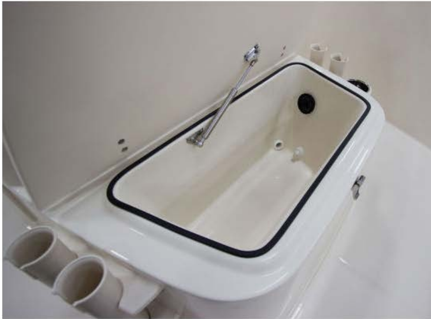
Located under the forward console seat, the standard 11-gallon (41.6 L) insulated raw water livewell with light and overboard drain.
