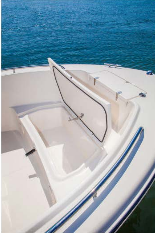
This 89 quart (84 L) fishbox is insulated and has a piston support strut and an overboard drain. Ice will last longer due to the gasketed lid.
