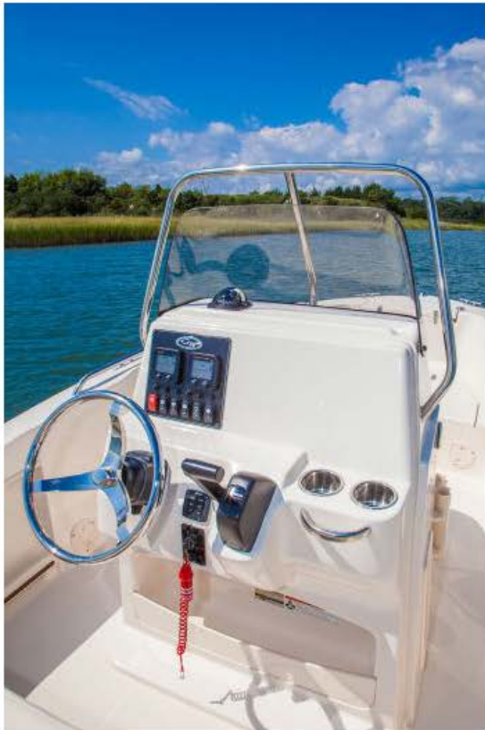
The Fisherman 180's helm console comes standard with a stainless steel wheel, a large electronic mounting area, an acrylic windshield and grab rail.
