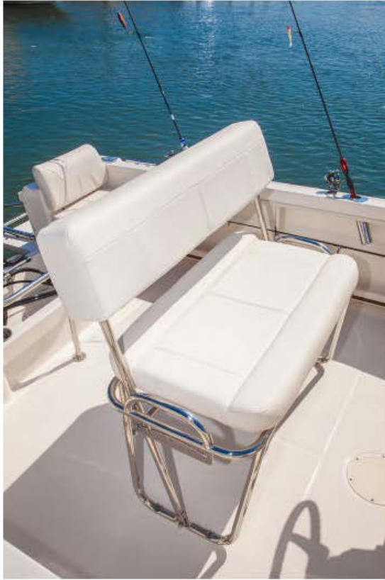
The helm's bench seat has a reversible back with a stainless steel frame.
