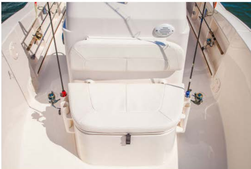
The console seat has everything handy for an angler: 2 rod holders on each side, 4 stainless steel trolling holders, 2 horizontal racks with gasketed tubes, as well as a cooler underneath the seat.
