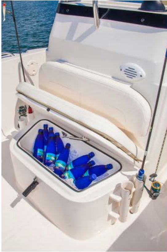
The console's front 45-quart ice box also includes piston support and has rod racks to the side.
