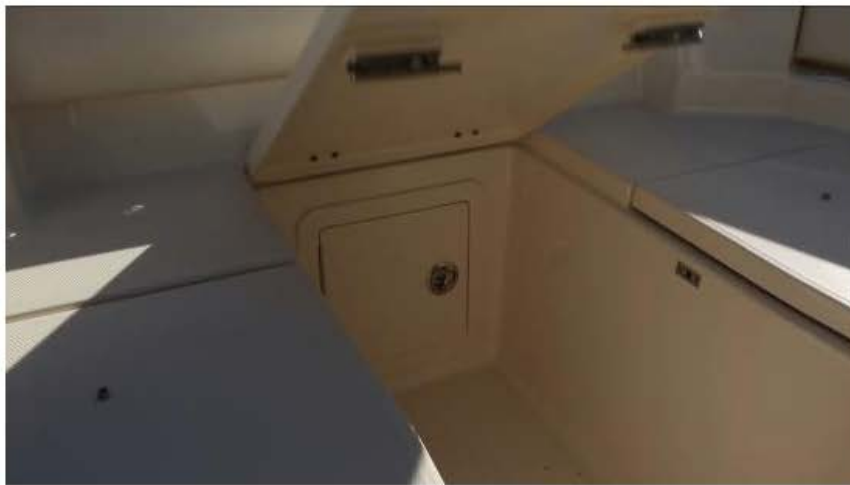
Under the forward platform is access to the rode locker.
