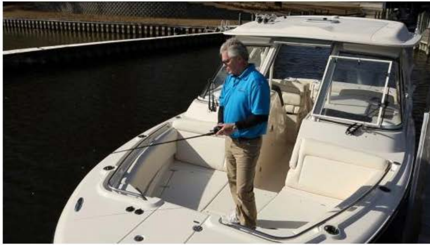
With the cushions removed, a casting deck is created.
