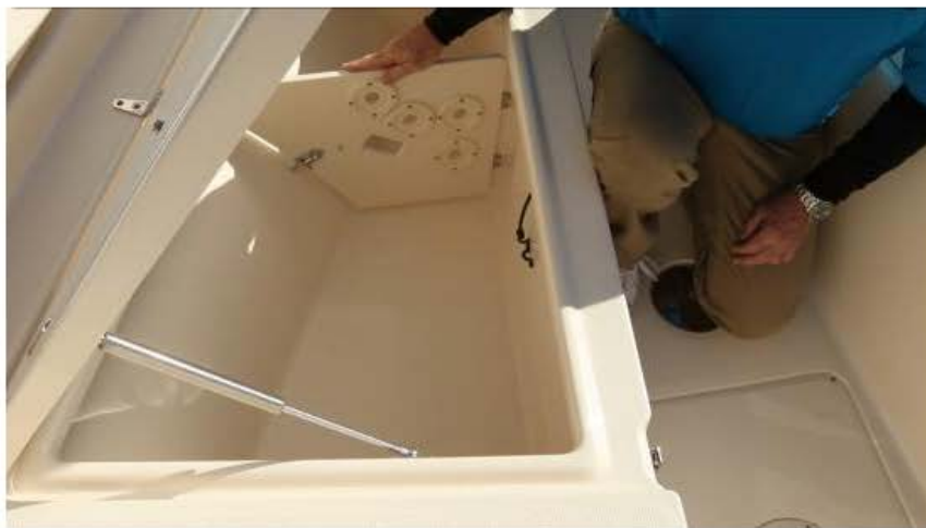
Under the port seating is open storage, or rod storage. This swing away panel, and another aft at the port console bulkhead, facilitates switching between the two.
