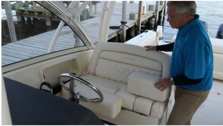
The helm seat includes separate flip-up bolsters.
