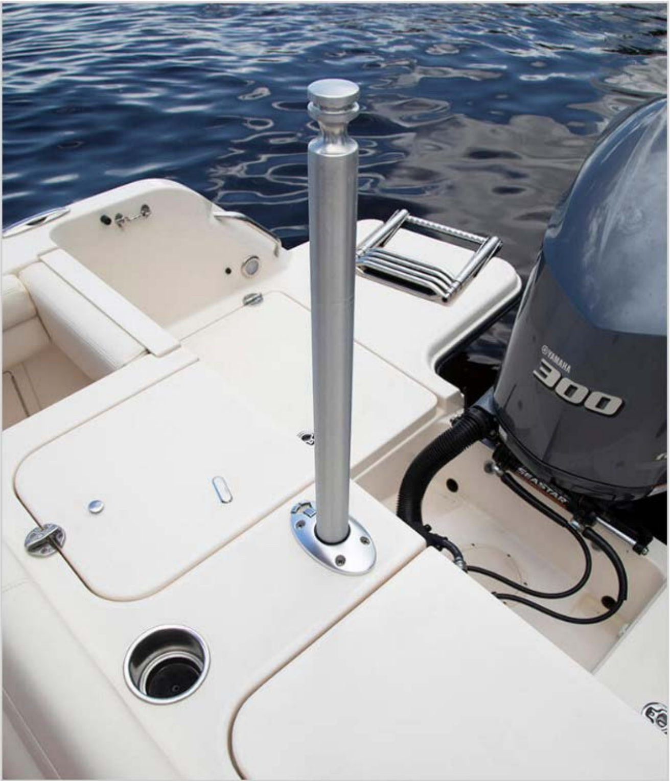
If tow sports are on the menu this retractable ski bit has you covered.
