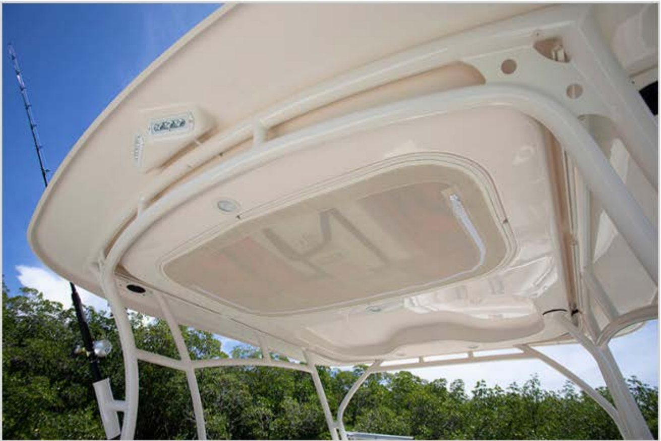
A hard top is useful for much more than providing shade as this fast access safety gear/PFD caddy demonstrates.
