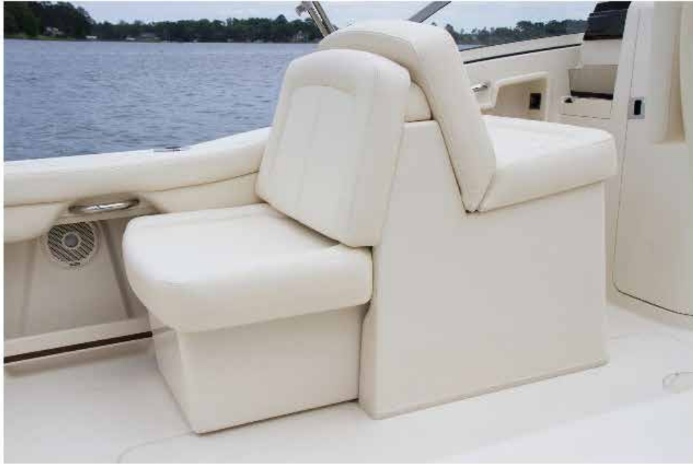
Deluxe companion seat configuration w/electromechanically extendable lounge seat. Note the corner door in the console which makes it easier to enter this small space.
