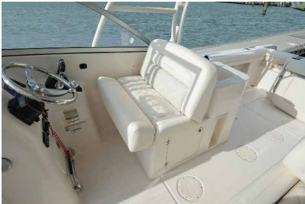
There is plenty of room between the rim of the wheel and the front of the seat, when moved back, to permit comfortable standing at the helm. The throttle pedestal is relatively horizontal which is a good thing. A chartplotter goes to the right of the wheel if you need one.
