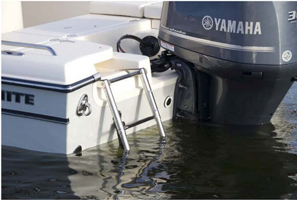
Behind the port side seat is a concealed re-boarding ladder.
