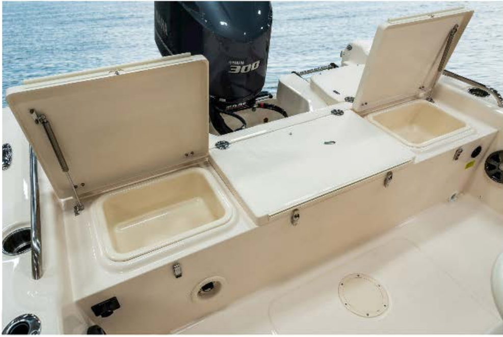
The transom seats lift to reveal storage bins port and starboard and an insulated, self-draining 51 quart (48.3 L) compartment that can be used as a fish box, beverage cooler, or for more storage.
