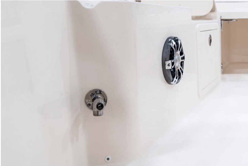
There's no shortage of stainless steel on the 251 CE, and that includes the raw water washdown spigot at the bow.
