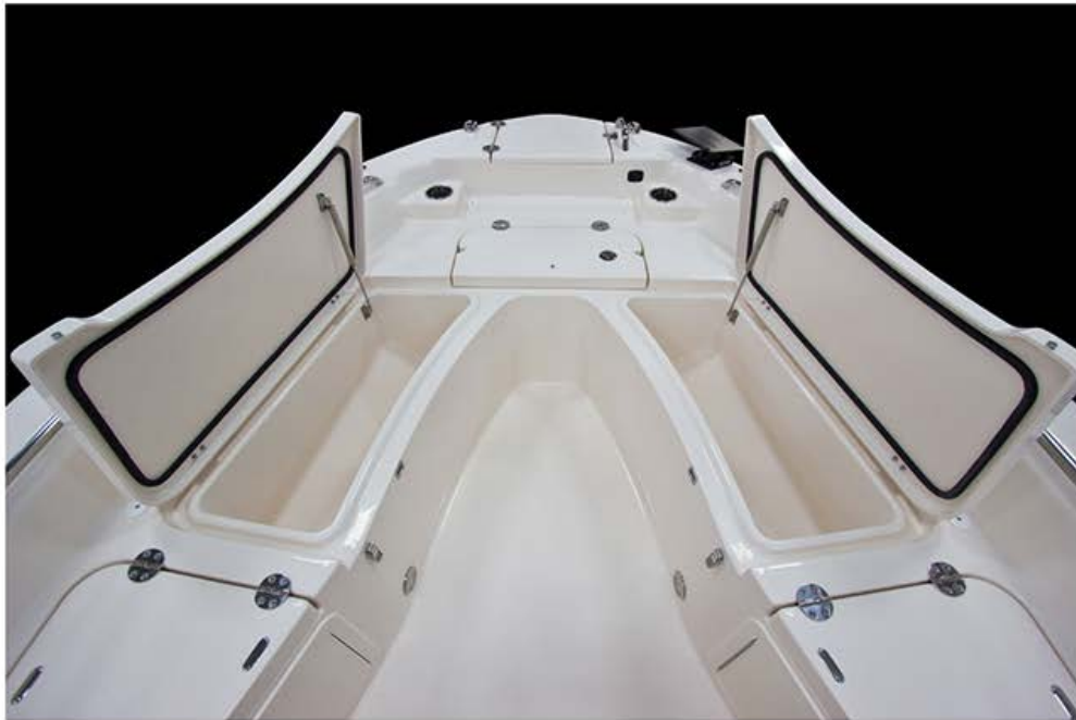
At the bow, there are two 74-quart fish boxes, port and starboard. Just behind are the lifting seat backs which create chaise seating.
