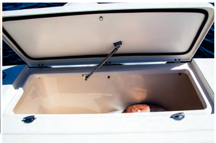
The genset is housed in its own soundproofed compartment in the transom; Right: A 274-litre insulated and drained fish bin dominates the transom.
