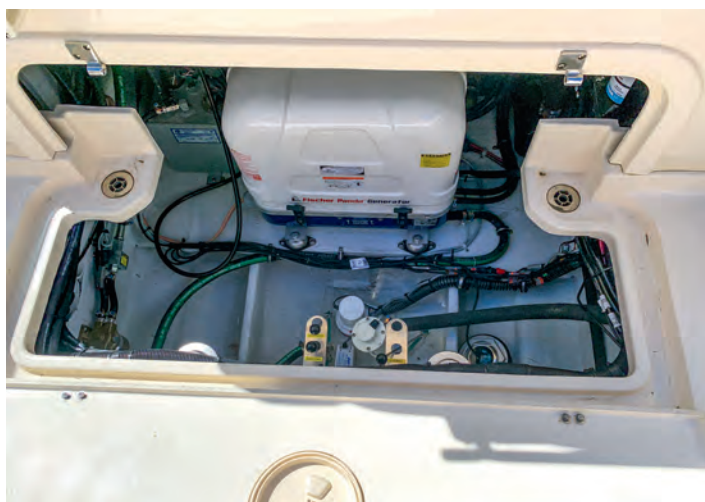
The genset is housed in its own soundproofed compartment in the transom; Right: A 274-litre insulated and drained fish bin dominates the transom.
