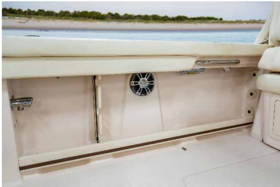
Raised toe rails are under the cockpit bulwarks and provide a little more security when leaning against the padded bolsters.
