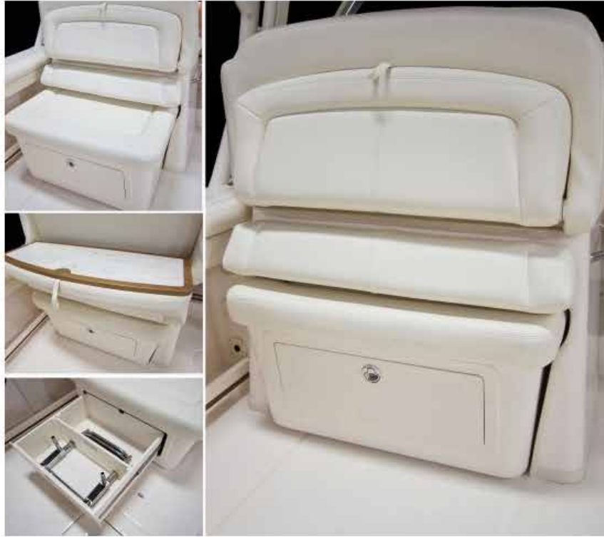
At the forward end of the cockpit is an electrically-actuated sliding cockpit bench seat with storage below.
