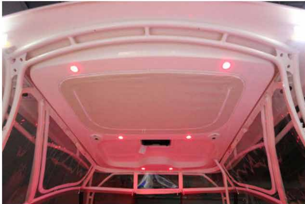
Night vision is spared with the tri-color LED lights. Select red, white or blue depending on the need.
