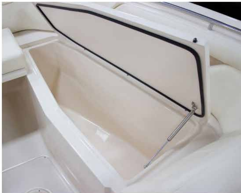
When the transom fishbox is full, go ahead and load up the bow one. Its 230-quart (218 L), insulated and has an overboard drain.
