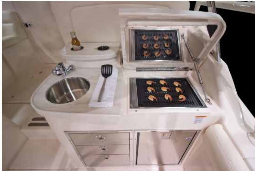
A wet bar presents a classy look with a combination of stainless steel and Corian. Seen here is the optional grill and below are stainless-steel storage drawers and a cockpit refrigerator.
