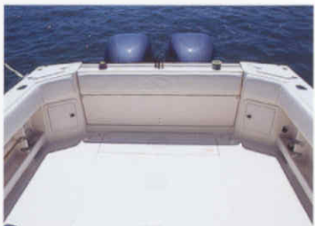
Aft cockpit with fold down motorwell bulkhead, aft deck lift out boxes, and optional cockpit bolsters
