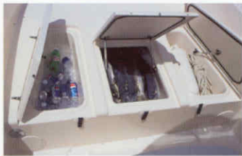
Casting platform with insulated bow fish boxes with overboard drains
