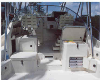
Cockpit forward with port insulated fish box, rigging station, sink, lockable tackle drawers and bulk storage
