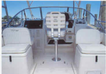
Helm area with removable seat backs and vertically and horizontally adjustable helm chair
