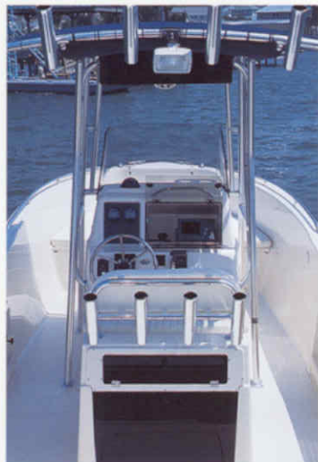
Cockpit forward with optional T-top and lean bar with tackle and bulk storage
