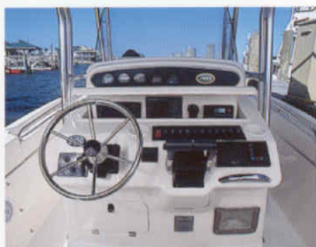
Helm console with electro-mechanically operated lockable electronics enclosure
