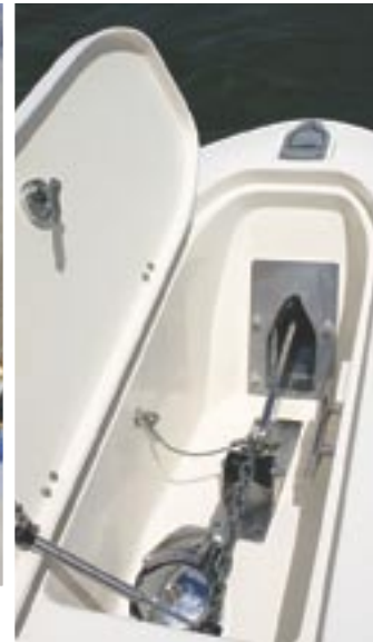
Anchor locker with windlass
