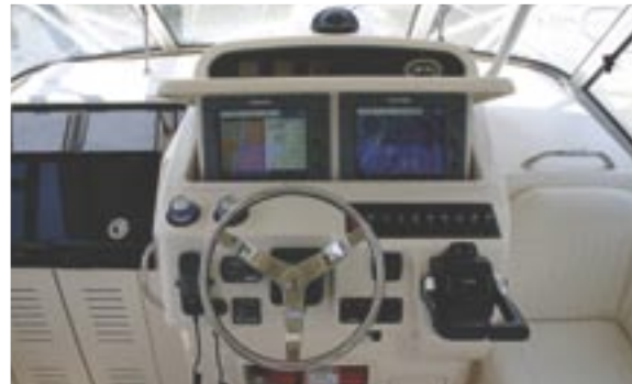
Helm station with electromechanically operated lockable electronics enclosure
