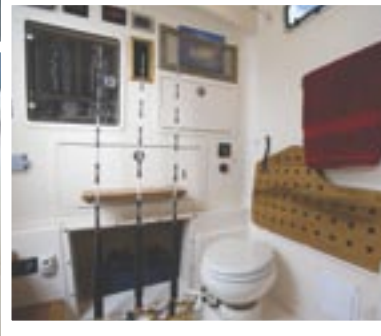
Lockable console interior with stand up head, shower, sink, rod storage, bulk storage and electrical access
