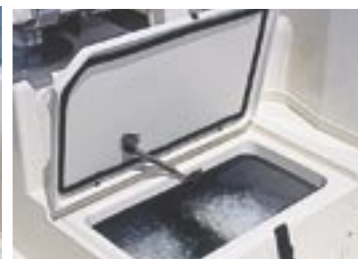
158-qt. starboard insulated fish box with overboard drain
