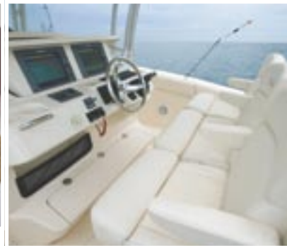
Center helm lean bar with three deluxe sliding seats and footrest, electromechanically operated lockable electronics enclosure
