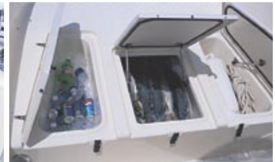
Insulated bow fish boxes with overboard drains
