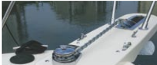
▲ Bow pulpit shown with anchor windlass option
