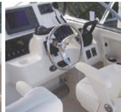
Helm station with electronics flush mount area
