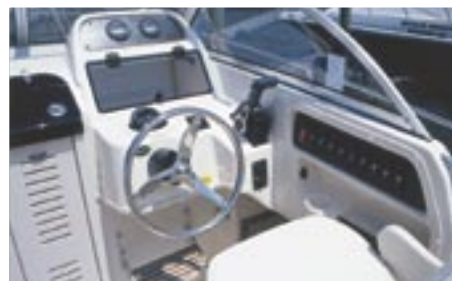
Helm station with lockable electronics box
