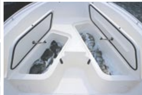
Insulated bow fish boxes with overboard drains
