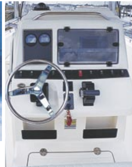
Helm station with lockable electronics box
