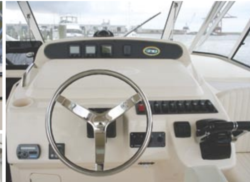
Helm console with electromechanically operated lockable electronics enclosure
