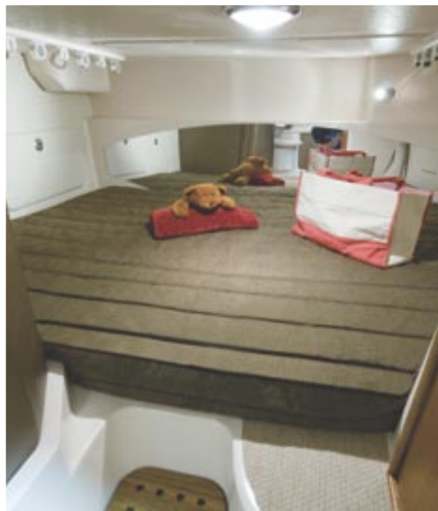
Aft berth includes 56" x 84" sleeping area with privacy curtain, teak foot well, teak hanging locker with cedar lining, bulk storage, six rod holders.
