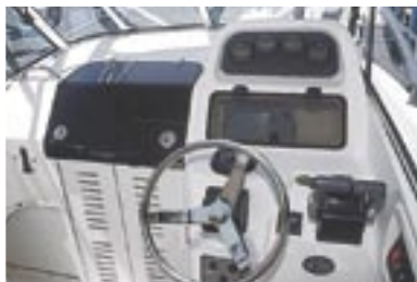
Helm station with lockable electronics box
