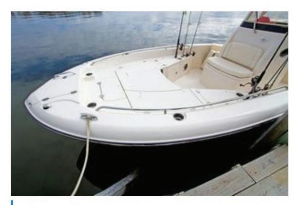
Grady's 251 Coastal Explorer features a sharp entry with some significant bow flare, while keeping fore and aft decks to appeal to inshore anglers.
