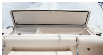
Above: Padded coaming bolsters cushion Capt. Sean Garrison's legs as he battles a strong fish. Right: The refrigerated fish locker features a divider to separate items such as frozen bait from your catch.
