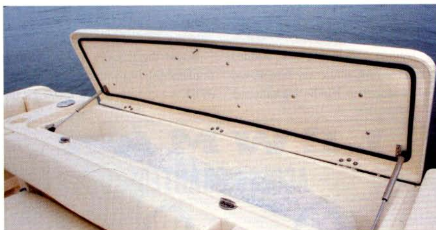
This transom fish box is huge and features a gasketed lid and gas struts to keep it open as you slam in a trophy-sized game fish. That's what the Grady-White people had in mind when they designed this fast express cruiser but the boat is very adaptable to many other uses, especially with the new enclosed hardtop.
