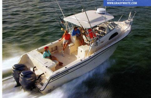
COCKPIT GEAR: Later models of the Marlin were built with a bench seat aft, a live well and a tackle station.
