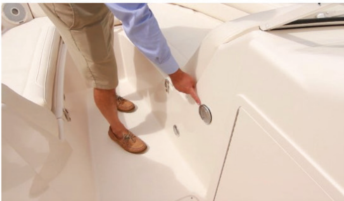
The test boat had the optional fresh water tank with the fill located in the forward inboard side of the starboard console.
