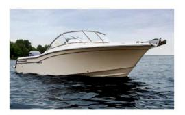
The 23-footer rides Grady-White's SeaV2 variable deadrise hull (20 degrees at the transom). It can be powered with a Yamaha F250 or F300. With an F300, the boat tops out at 44 mph and gets about 3 mpg at 26 to 28 mph. At 41 mph, mileage dips to 2 mpg. With an F250, the boat hits 43 mph wide open and cruises at 26 mph with a mileage rating of 2.7 mpg. The F250-powered boat also gets 2 mpg at 41 mph but at a higher rpm of 5,500. Fuel capacity is 115 gallons.
