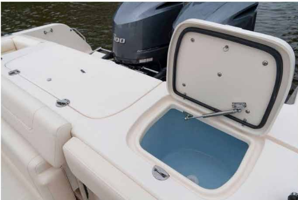
The livewell has a 32-gallon capacity.
