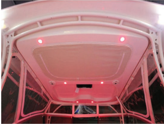
Night vision is spared with the tri-color LED lights. Select red, white or blue depending on the need.
