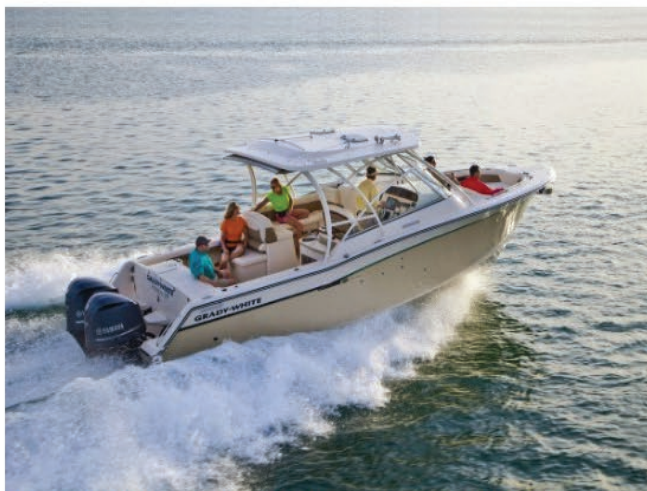
The Grady-White Freedom 335 has a LOA of 33'6" (10.21 m), a beam of 11'7" (3.53 m) and a hull draft of 26" (66 cm).
