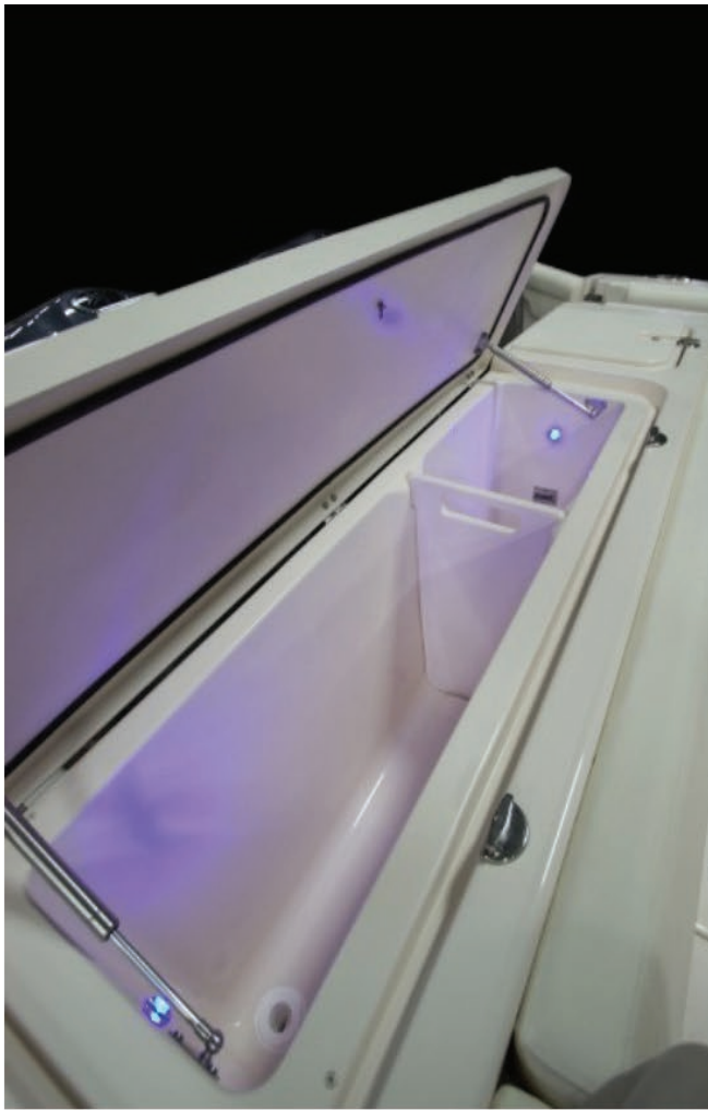
A cooler can be swapped out for this livewell that is next to the insulated fishbox. Frankly, when in party mode both can hold plenty of ice and drinks.
