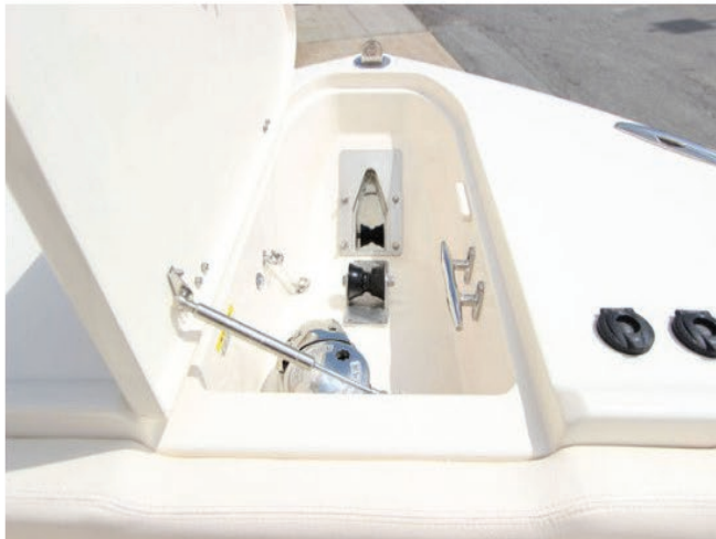
The anchor hatch is back gelled and held open by a gas assist strut. The switches to control the windlass are just alongside.
