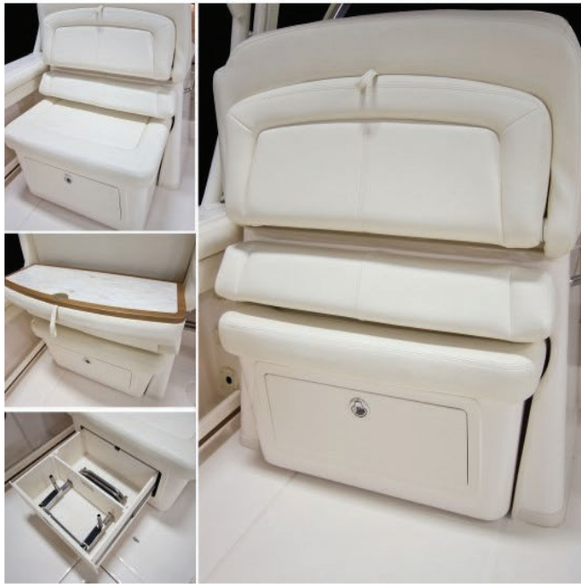
At the forward end of the cockpit is an electrically actuated sliding cockpit bench seat with storage below.
