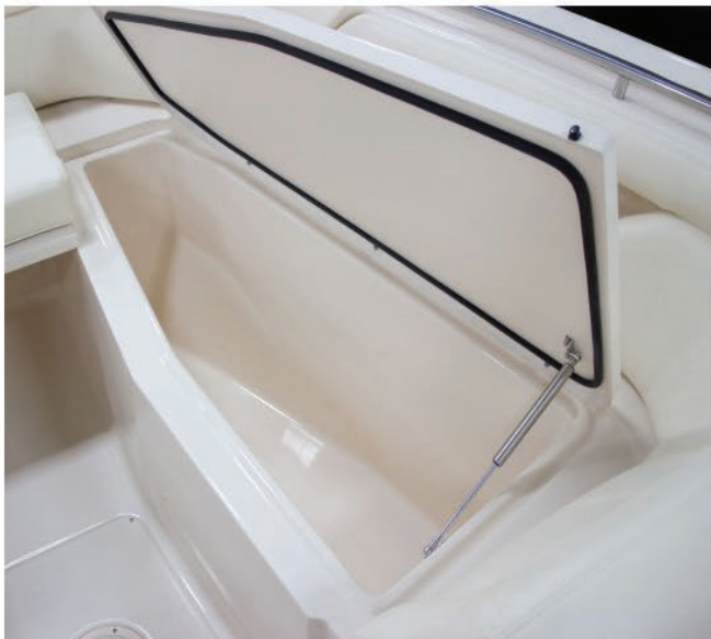
When the transom fishbox is full, go ahead and load up the bow one. Its 230-quart (218 L), insulated and has an overboard drain.
