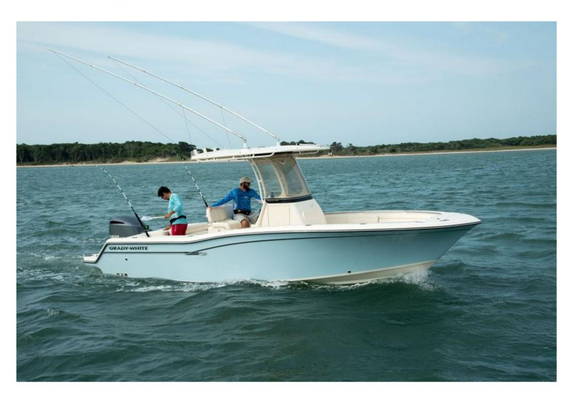
LOA: 23 ft. 7 in.; Beam: 8 ft. 6 in.; Draft: 1 ft. 6.5 in.; Deadrise: 20 deg.; Max Power: 300 hp Courtesy of Grady-White Boats
