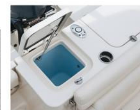
The transom houses a sizable livewell, as well as a 160-quart insulated fish box.
