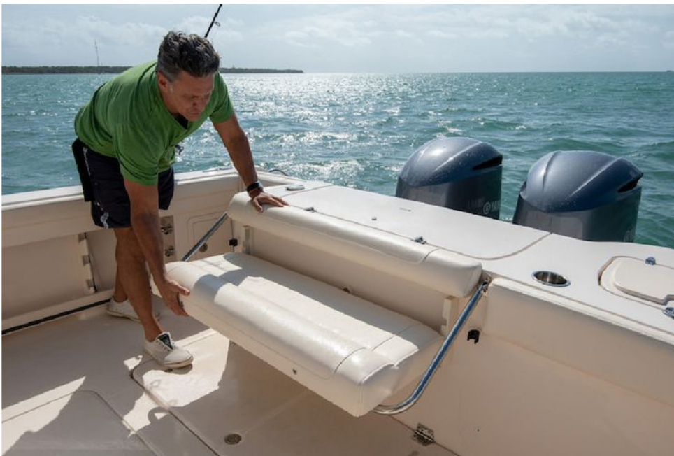
The fold-down benchseat tucks away when you want cockpit space for fighting fish. Courtesy Grady-White
