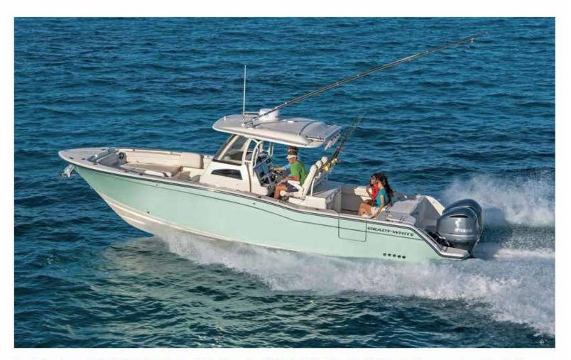
Specifications: LOA 33 ft. 1 in.; Beam 10 ft. 9 in.; Dry Weight 8,500 lb.; Fuel 327 gal.; Transom Deadrise 20 deg.; Max HP 700 hp. *Grady-White*
