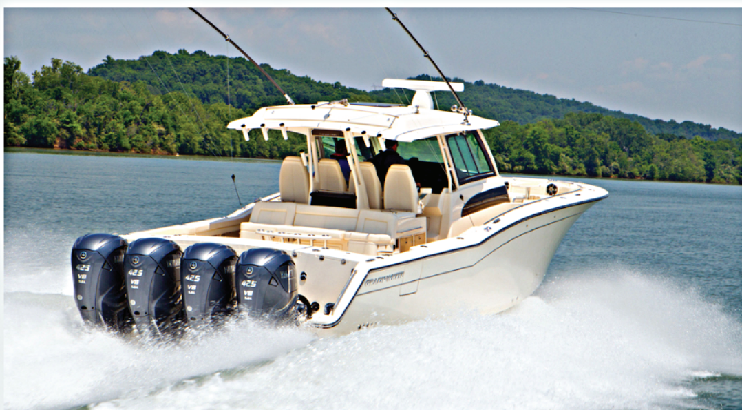
Quad Yamaha XTO Offshore 425 outboards pushed the 35,000-pound Grady-White Canyon 456 to 58 mph and made it handle like a dream.
